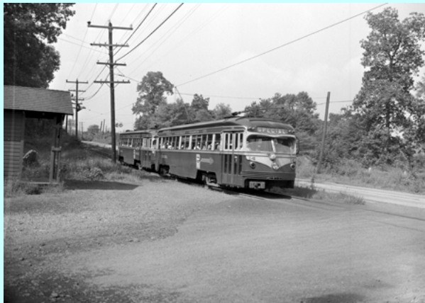
Figure 4 - St. Louis Car Co.- built Red Arrow 11-24 series cars on West Chester Pike before end of rail service in June 1954. Most of the line was side-of-the-road trackage.
