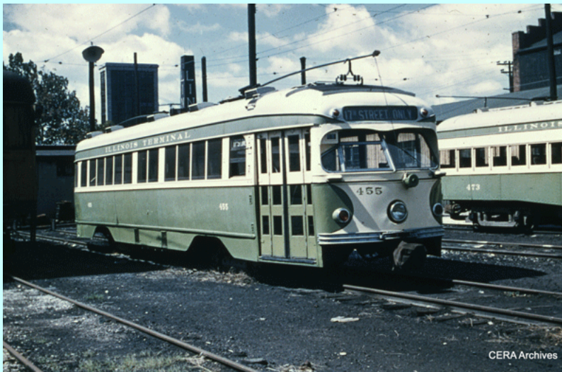
Figure 5 - The St. Louis PCCs built for Illinois Terminal for its St. Louis, Mo., to Granite City, Ill., run were unique in having only front doors. IT 455 at Granite City in September 1953. (Photographer unknown - CERA Archives)
